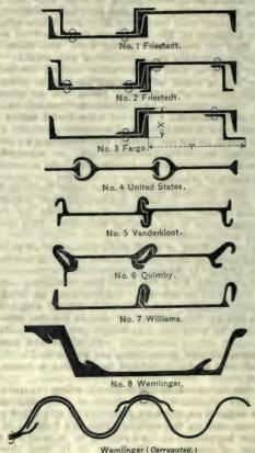
Fig. 3.—Representative Steel Sheet Pile Sections.
